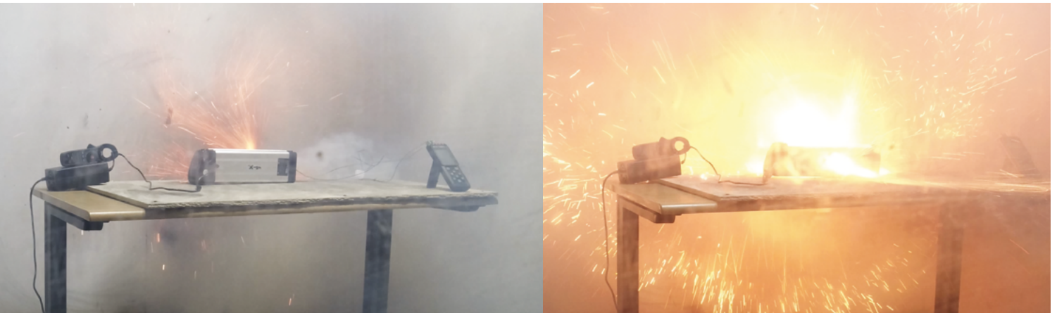
Figure 30: Photos of test sample during a thermal runaway event after being incorrectly charged.
