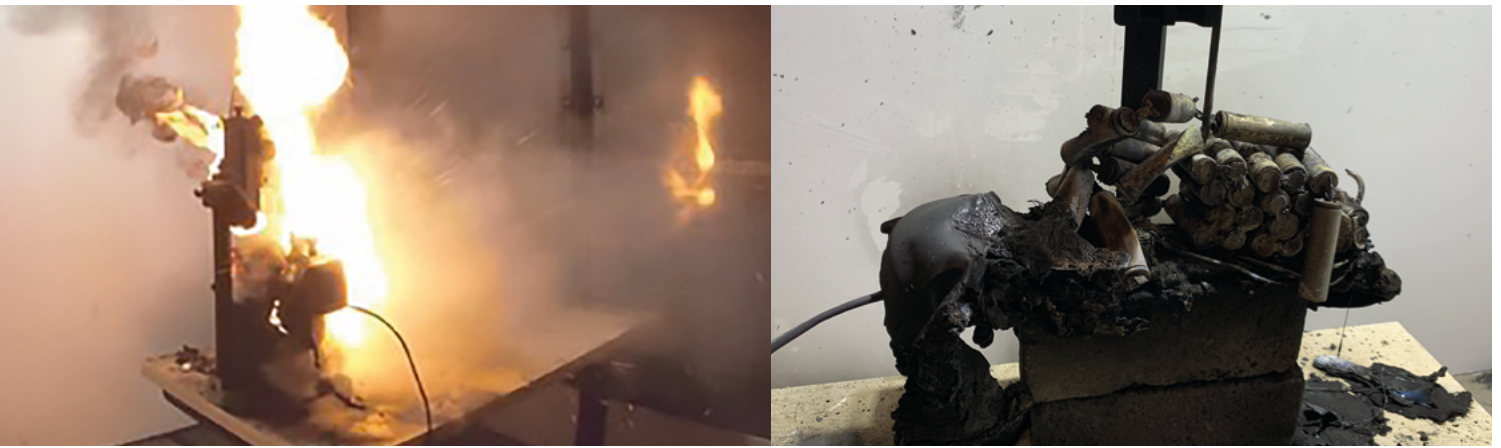
Figure 29: Photos of test sample during and post thermal runaway event from a simulated nail penetration test.
