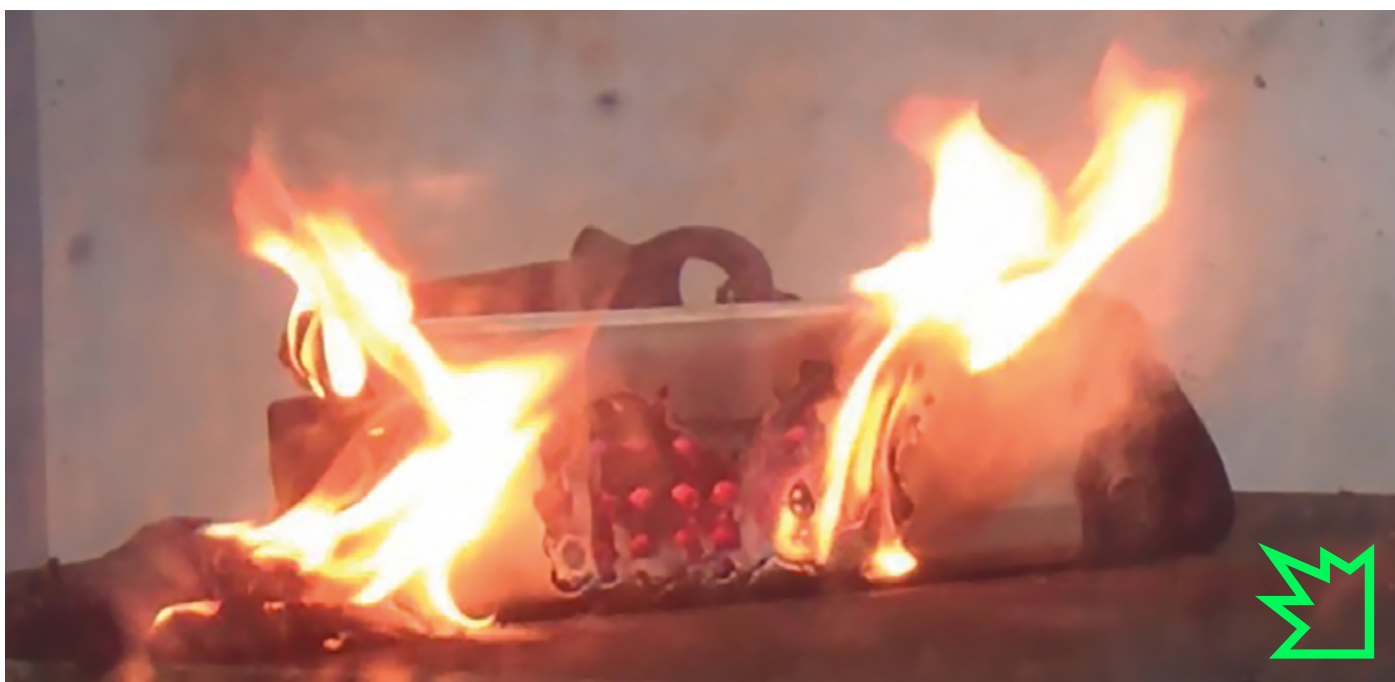
Figure 18: E-bike battery following a thermal runaway event caused by overcharging.
