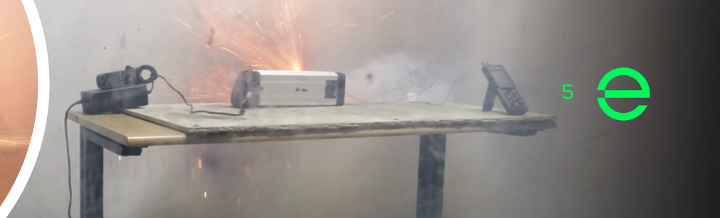
Figure 2: Photos of test sample during a thermal runaway event after being incorrectly charged.
