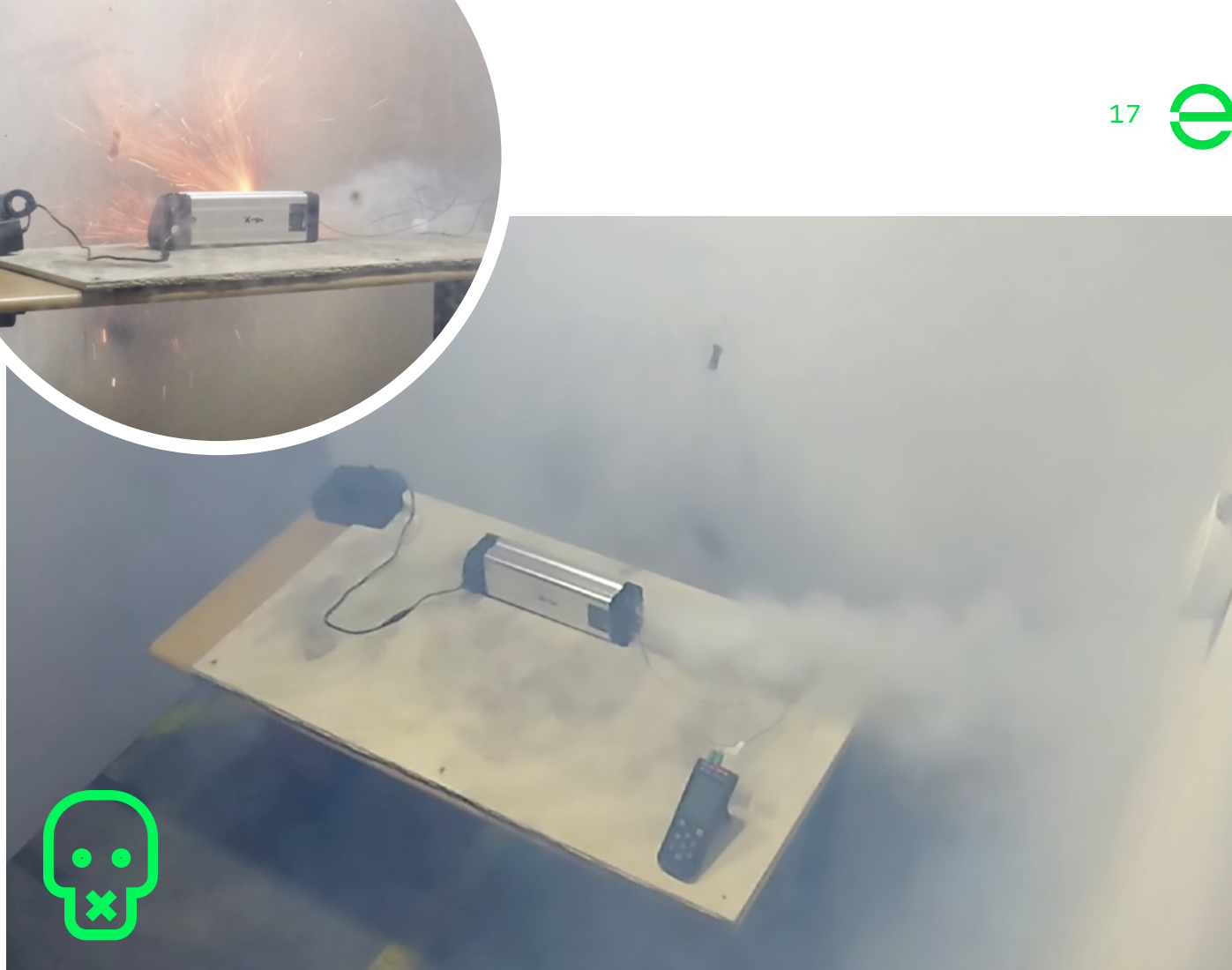
Figure 11: ©ESF Onset of thermal runaway – venting of a vapour cloud of highly flammable and toxic gases.
