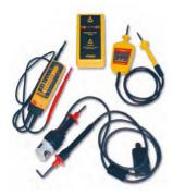
The test lamp or voltage detector should be proved to be working on a compatible proprietary proving unit, or a known live source, or an in-built test function before and after use.
