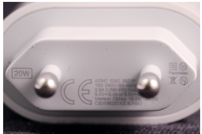
Figure 17: Example of manufacturers placing the CE mark on an unsafe charger that does not meet the requirements of the European Low Voltage Directive and marking the product with certification marks to suggest that it has been tested and approved by a third-party test house (Sample 65).
