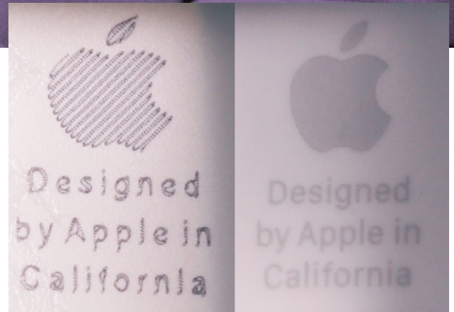
Figure 19: Side by side markings comparison for counterfeit (left) and genuine (right).
