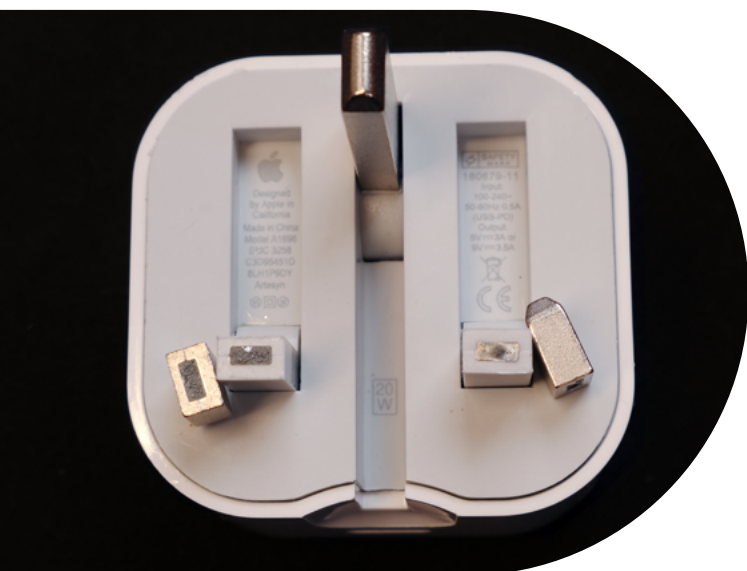
Figure 09: A counterfeit Apple charger that failed the mechanical strength test.
