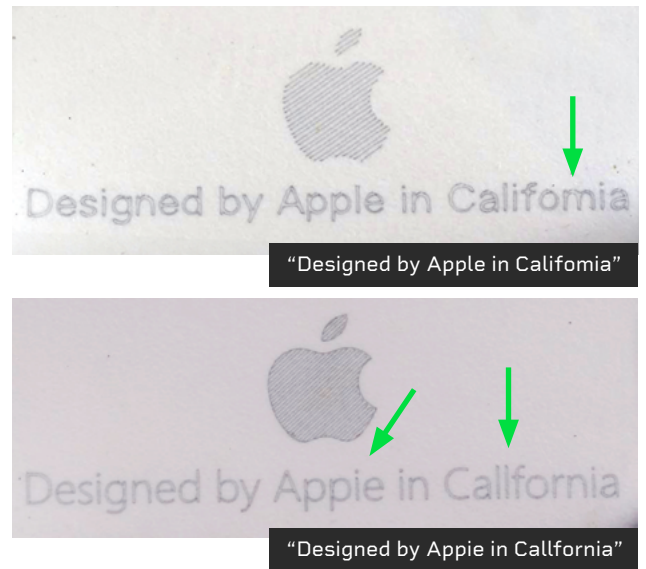
Figure 20: Examples of merged markings and spelling mistakes on counterfeit Apple chargers.
