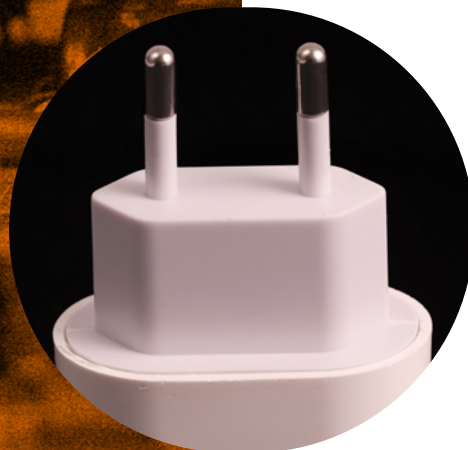
Figure 05: Example of imitation charger sold with no markings.
