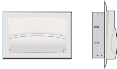
Typical flush-mounted consumer unit
