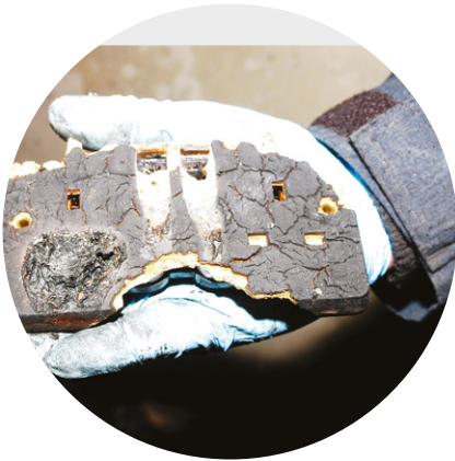
The effect of fire on a socket-outlet (Photo courtesy of Greater Manchester Fire & Rescue Service)
