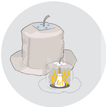
Typical fire hood for a downlighter
