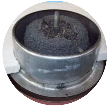
Fire rated Ceiling Air Valve sealed after a fire Photos courtesy of Tenmat Ltd
