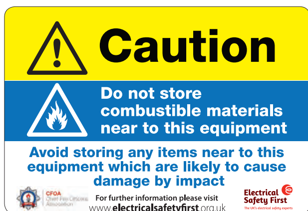
Label warning against storing combustible materials near to electrical equipment
